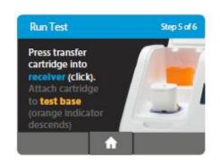
Caution: The orange indicator should be observed closely. If the orange indicator does not fully rise, the Transfer Cartridge may not collect enough sample.
