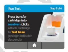
Caution: The orange indicator should be observed closely. If the orange indicator does not fully rise, the Transfer Cartridge may not collect enough sample.
